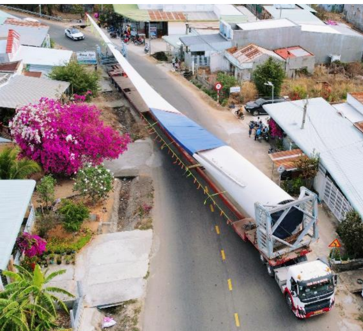
风力发电机叶片：L71m x W3.6m x H4.48m
